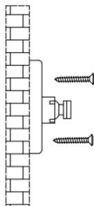
Mount the bracket with the included screws as shown above. Then place the motion detector in the bracket. Specify the right direction of the detection range of the motion sensor. Test the operation of the motion detector by putting it into testing mode which has been described at the former page.
